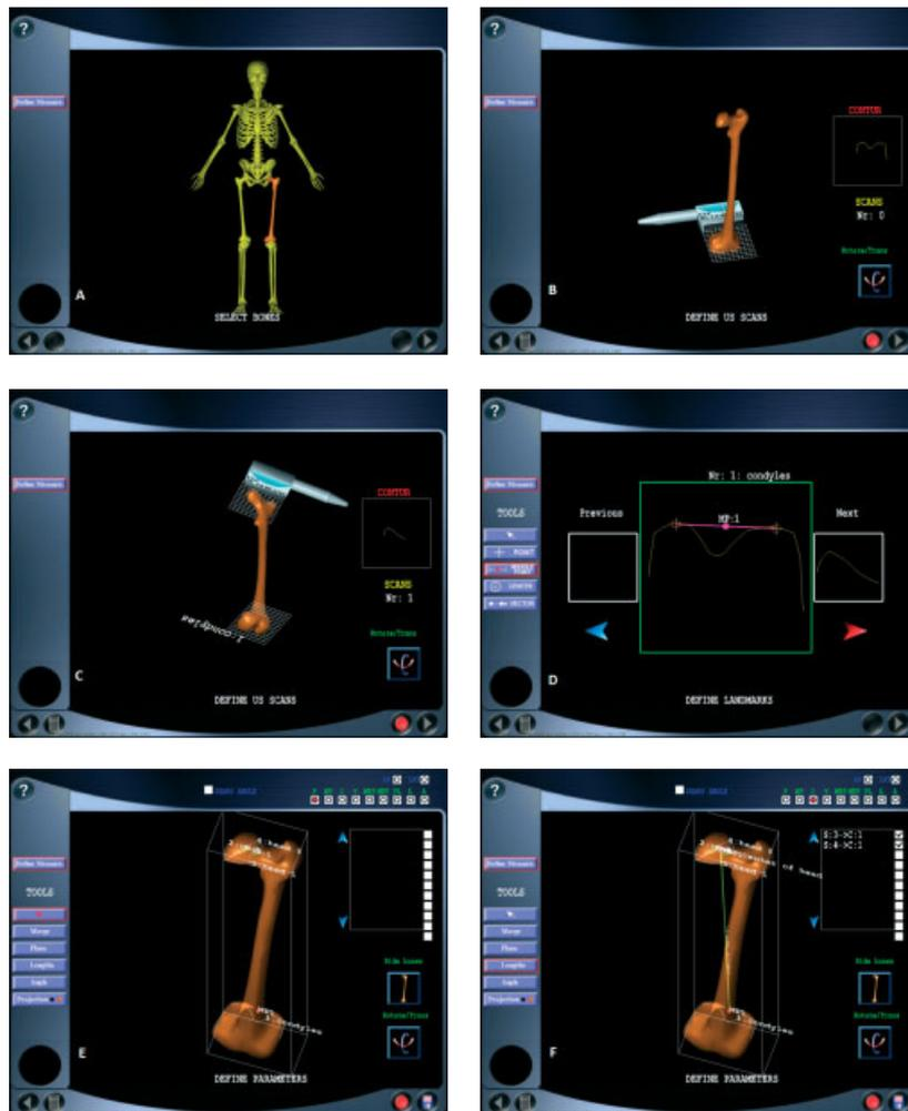
Figure 4. Definition of femur length measuring procedure template: (A) selection of bone (femur); (B) definition of probe position and virtual scan of condyles; (C) virtual scan of femur head; (D) definition of landmark (middle point between condyle points); (E) definition of length between femur head centre and knee centre; (F) 3D visualization of defined femur length
