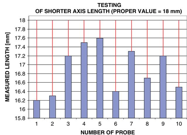
Figure 10. Results of measurement of volumetric object’s shorter axis
