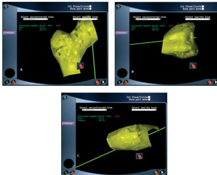
Figure 13. Results of ultrasound-based reconstruction of three regions of femur synbones (A – head, B – condyles and C – shaft)
