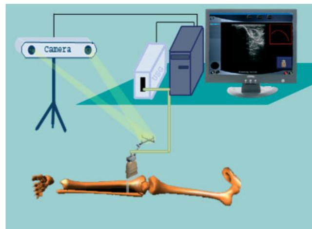
Figure 1. System for noninvasive bone measurements
