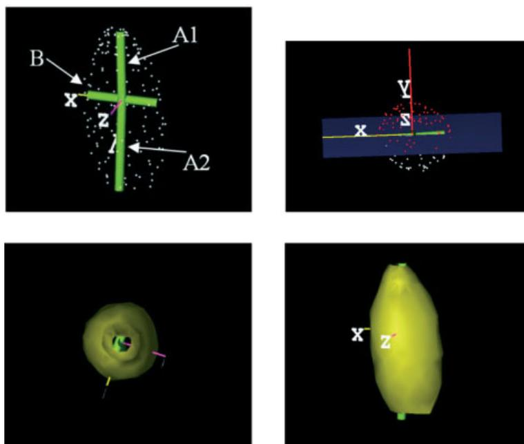
Figure 11. Volumetric object reconstruction: (a) cloud of points; (b) reconstruction procedure; (c) 3D views of reconstructed object
