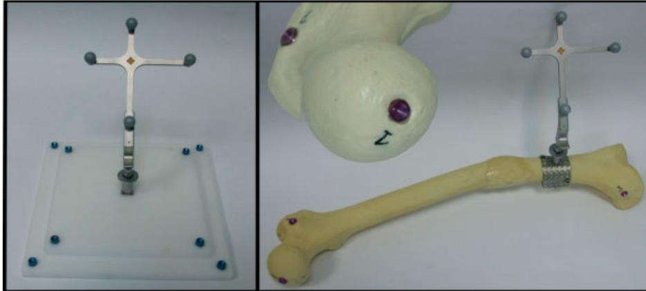
Figure 6. Measuring plate and one sawbone with mounted cones and reference rigid body
