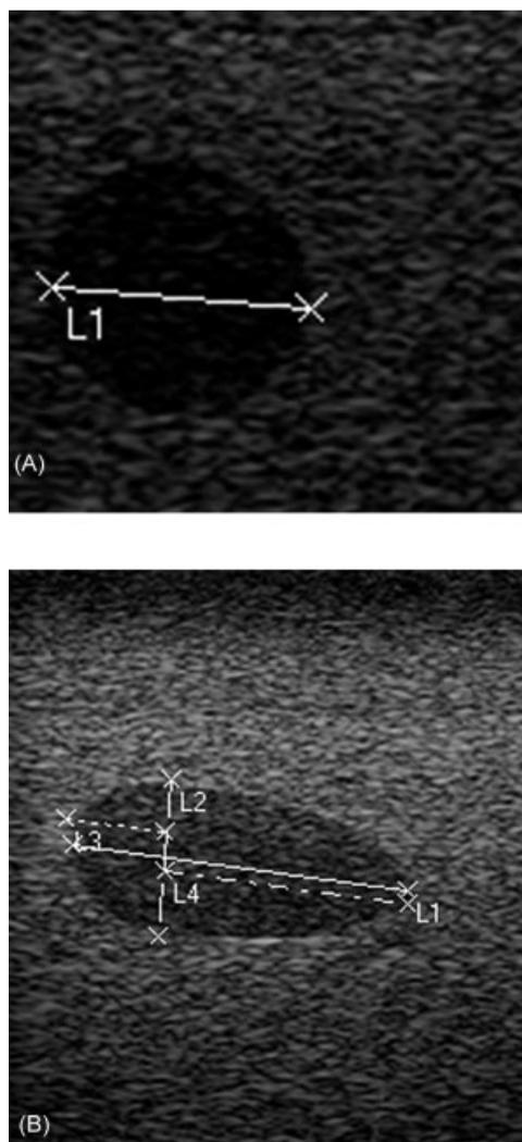
Figure 7. Scan of volumetric object: intersection is a circle and ellipse
