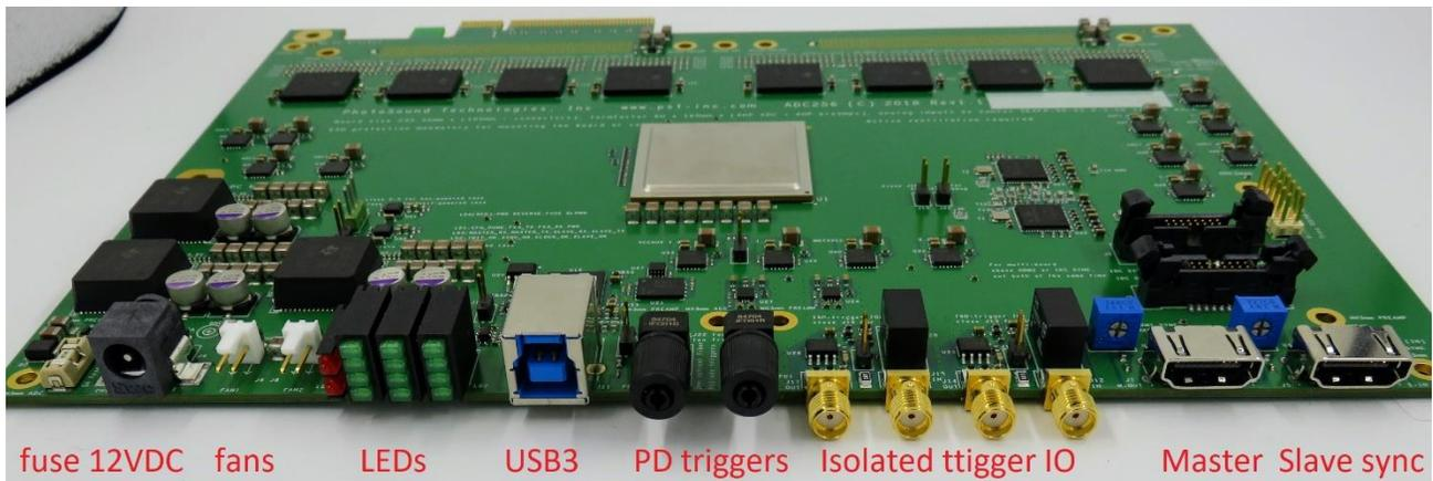
**Figure 1:** Bare ADC256 board with labeled digital IO connectors.
