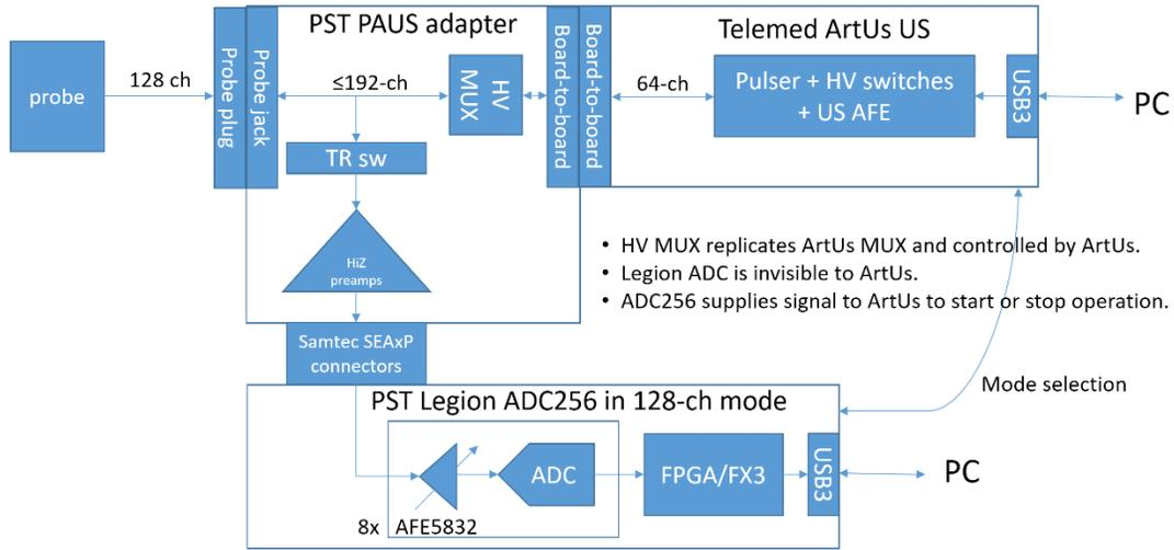
Figure 4: MolecuUS US and PA system block-diagram.
