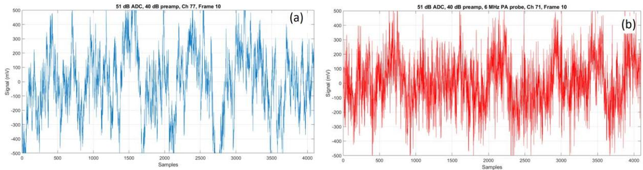
**Figure 2:** Noise traces from individual channels with RMS close to or equal to the average value. (a) 51 dB ADC + 40 dB preamplifier; (b) same amplification + PA probe with element capacitance 105pF, notice low frequency noise reduction.
