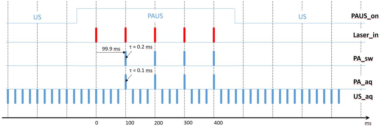
Figure 5: MolecuUS US-PA communication protocol with a 10 Hz laser. Frame rates up to 200 Hz are supported for PA applications.
