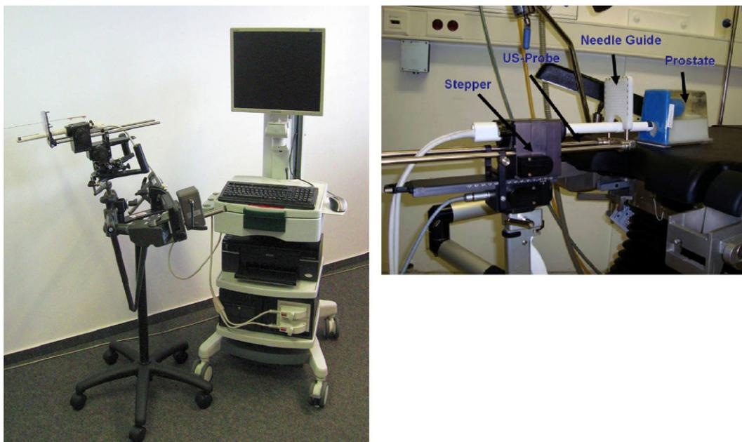
**Figure 1.** BiopSee system consists of personal computer with integrated US device and additional electronics to control position and orientation of US probe. Probe has custom biplane endorectal design and is placed on custom mechanical stepper. Device movement is tracked by 2 encoders with resolution of 0.1 mm and 0.1 degree.
