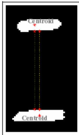
**Figure 6-11 Illustration of distribution of points for vertical distance measurement**
