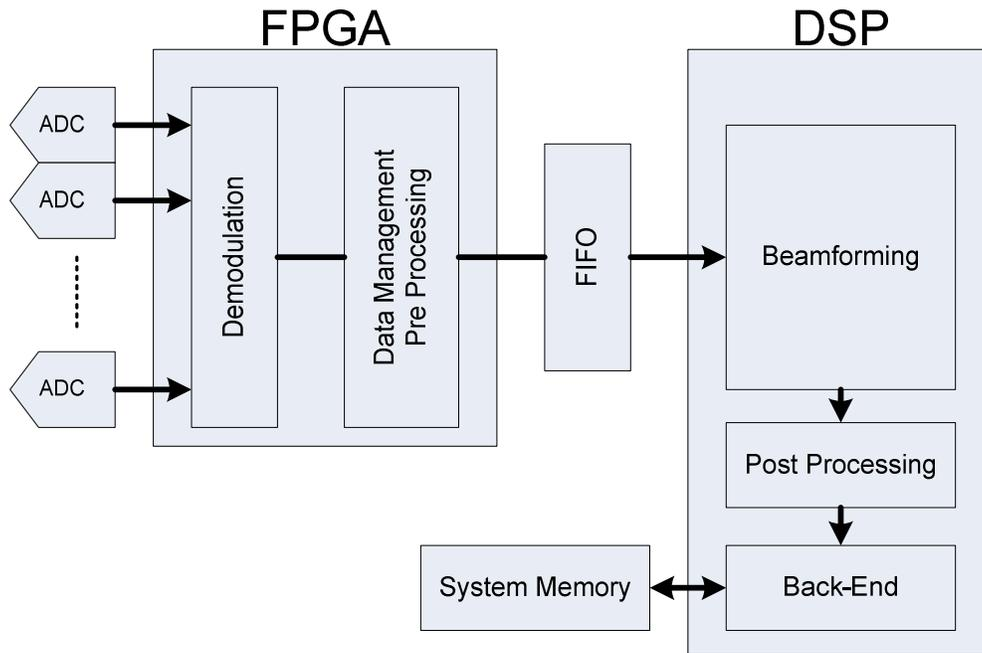
Figure 3-6 Ultrasound Signal Processing Process Diagram
