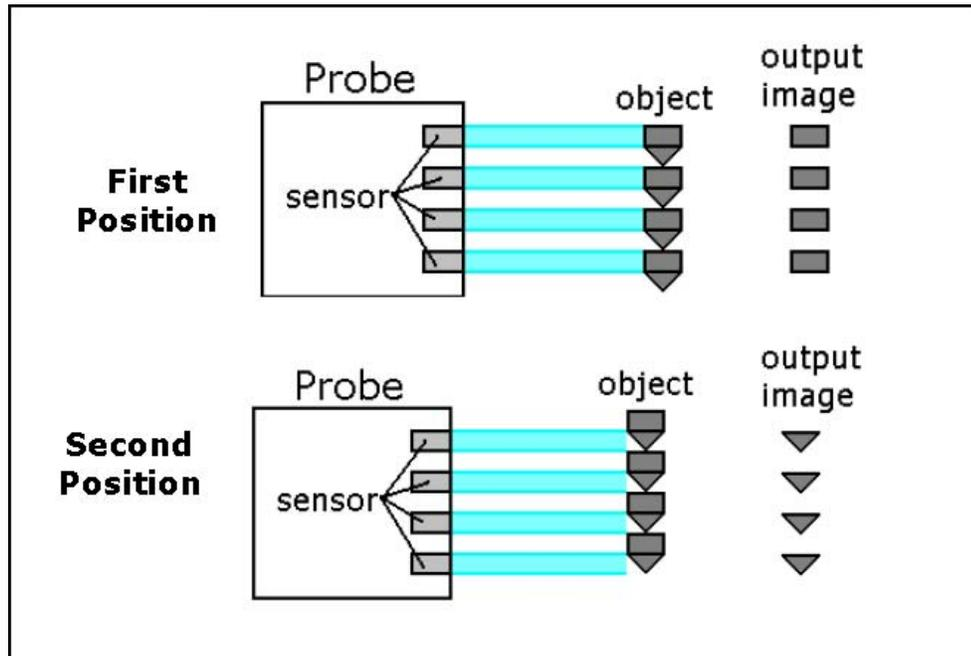
Figure 6-3 Image captured on first and second position
