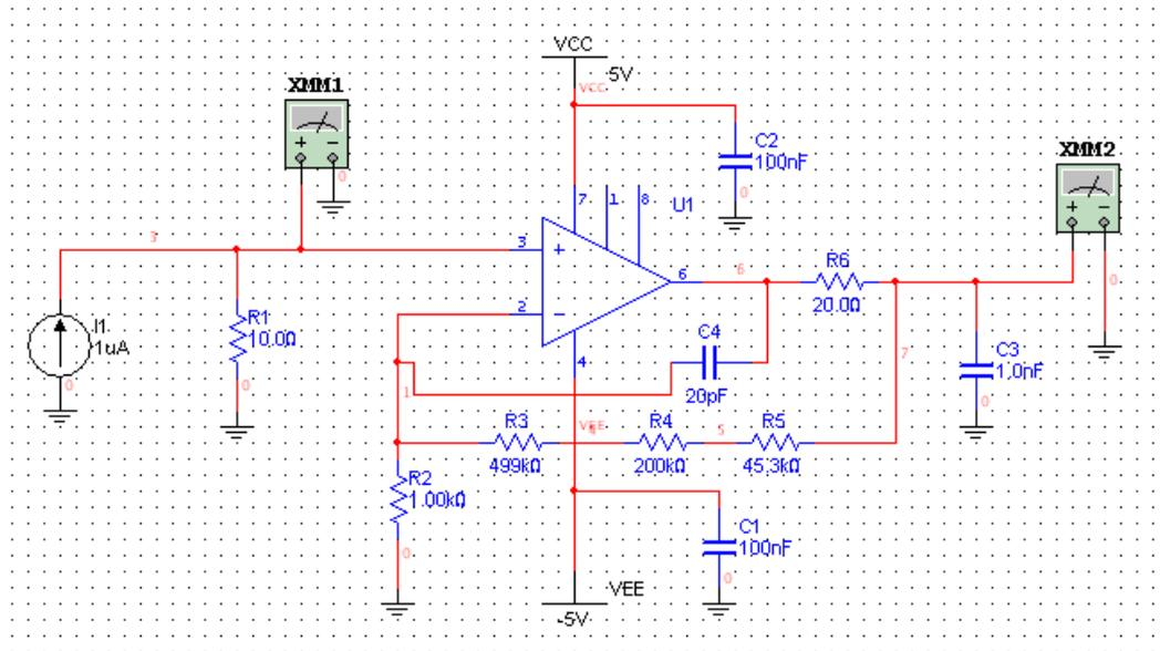
Figure 6-29 The amplifier circuit
