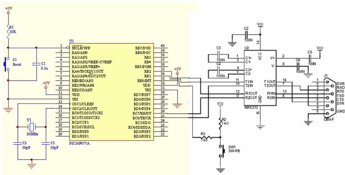
**Figure 6-34 The connection circuit between MAX232, RS232 and the PIC microcontroller**
