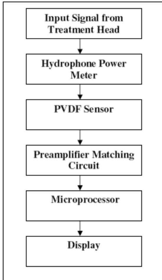
**Figure 6-16 Block diagram of the designed system**
