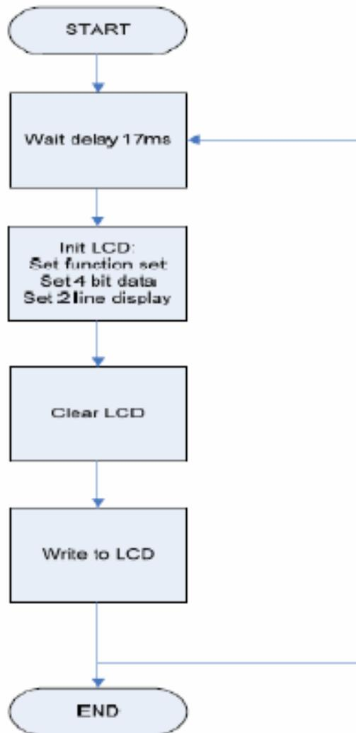
**Figure 6-24 LCD set up**
