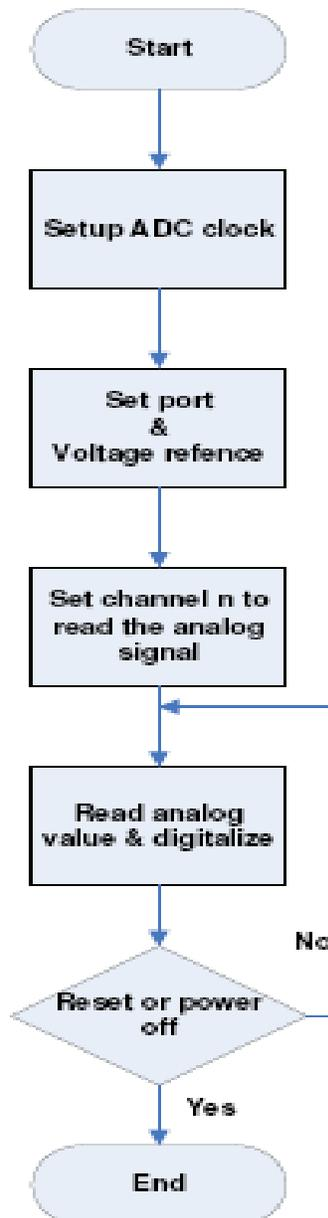
Figure 6-25 ADC setup
