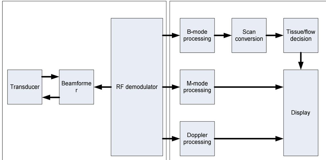
**Figure 3-2 Portable Ultrasound Block Diagram**
