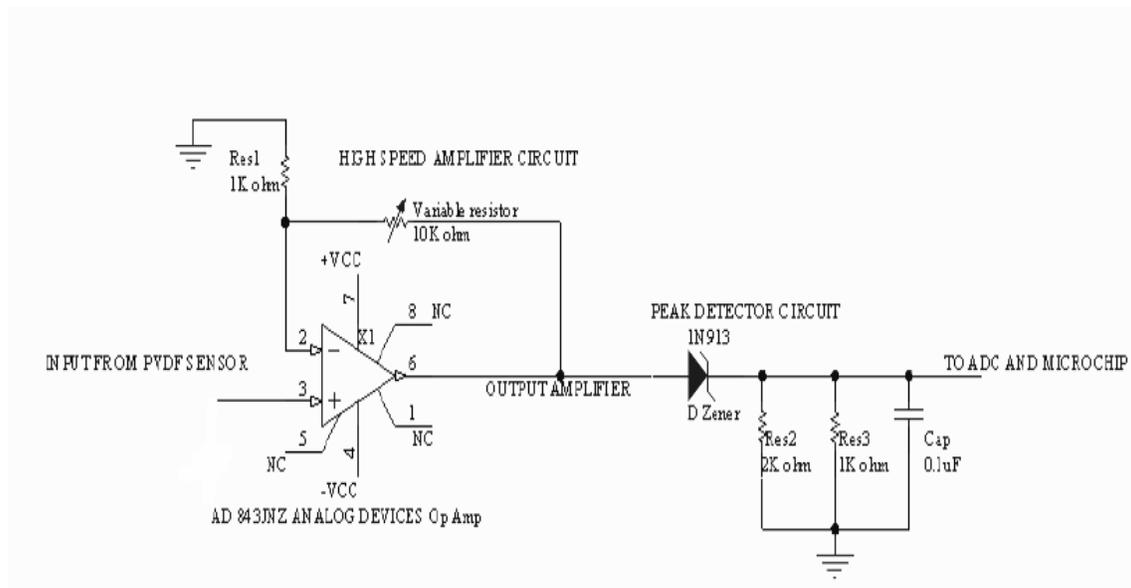
Figure 6-19 Pre-amplifier matching amplifier and peak detector schematic circuit
