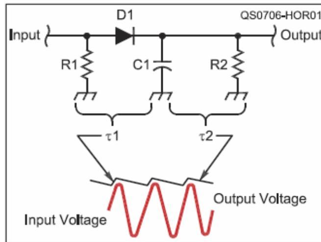
**Figure 6-22 Signal generated by peak detector circuit**
