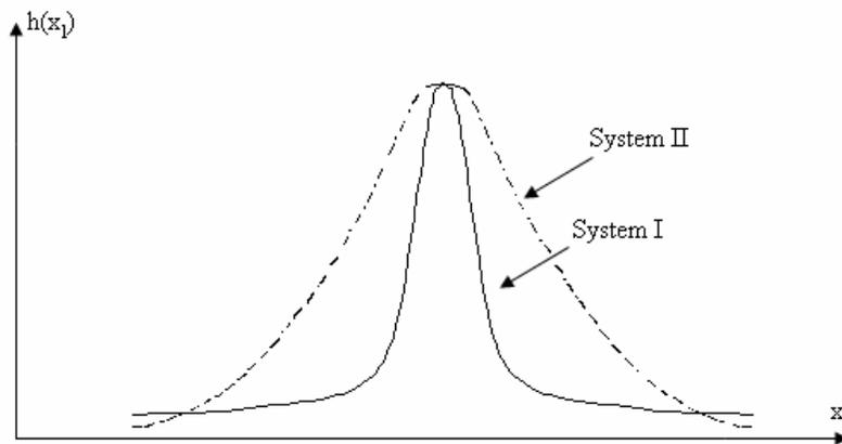
**Figure 5-1 Point spread function of two imaging systems represented by grey-scale distributions as a function of one spatial dimension. System I has a narrow point spread function and therefore better spatial resolution than system II**
