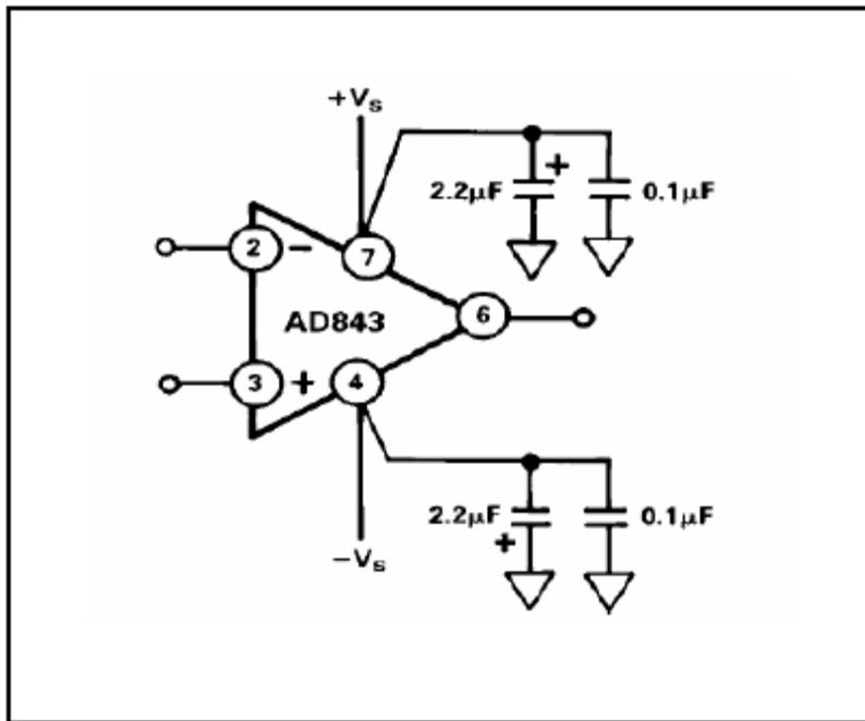
**Figure 6-21 Recommended Power Supply Bypassing for the AD843**
