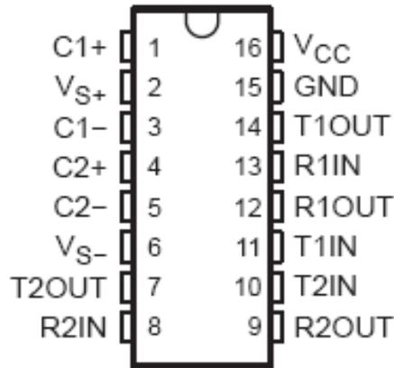
**Figure 6-33 The MAX232 schematic diagram**
