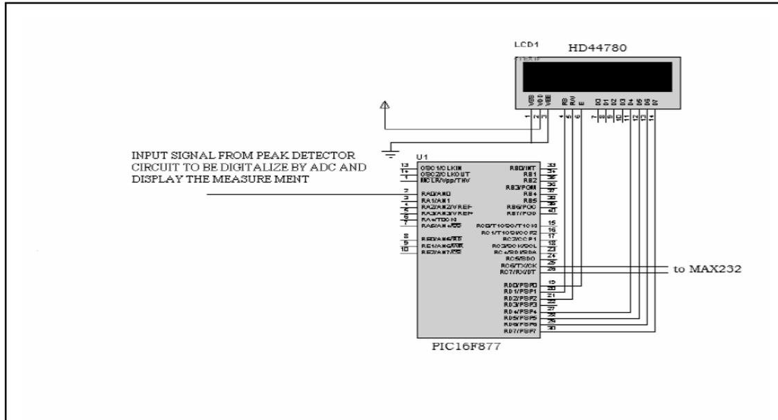
Figure 6-23 Connection between the microcontroller and peak detector circuit
