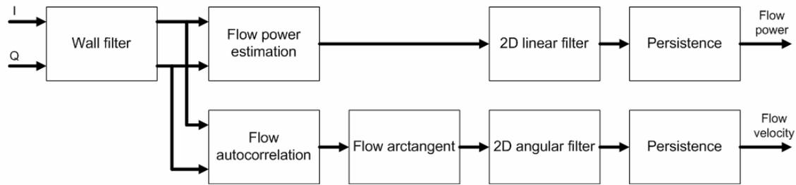
**Figure 4-4 Block diagram of color-flow processing**
