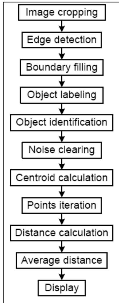
Figure 6-5 Flow of automatic measurement
