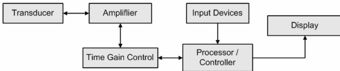
Figure 3-7 Ultrasound machine diagram block
