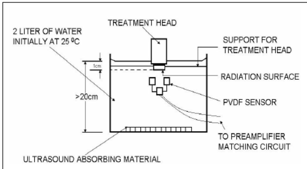
Figure 6-15 The designed of hydrophone
