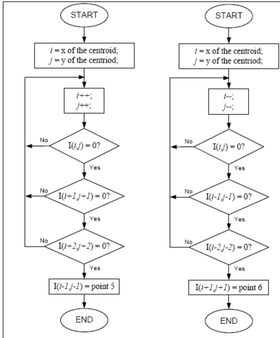
Figure 6-8 Iteration flow for point 5 and 6
