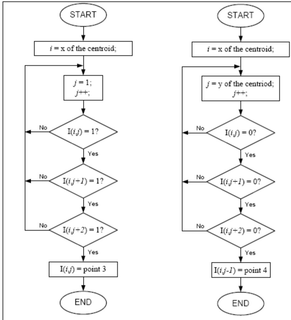
Figure 6-7 Iteration flow for point 3 and 4
