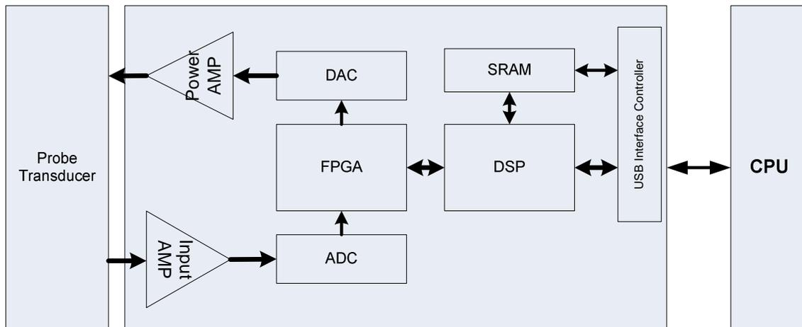
Figure 3-5 Block Diagram of Signal Processing Box of PC based Ultrasound
