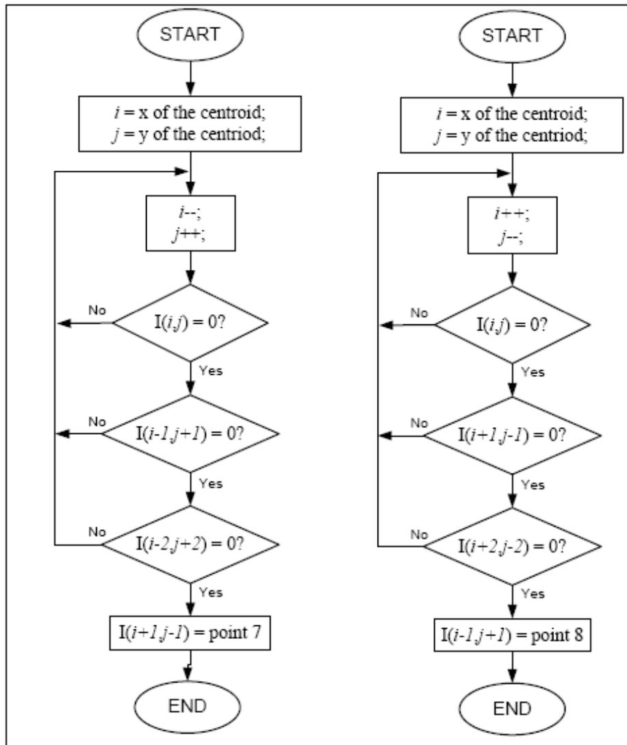
Figure 6-9 Iteration flow for point 7 and 8
