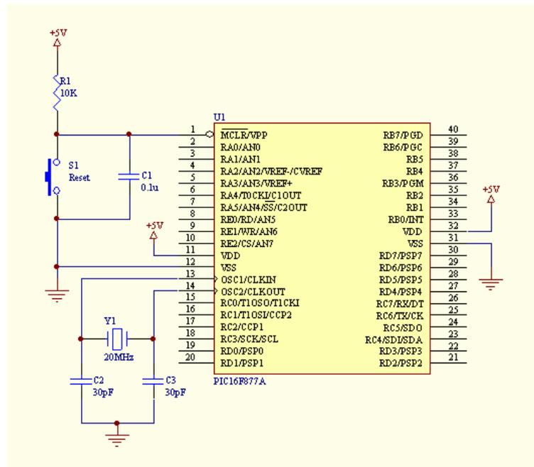
Figure 6-31 The PIC16F77A microcontroller circuit
