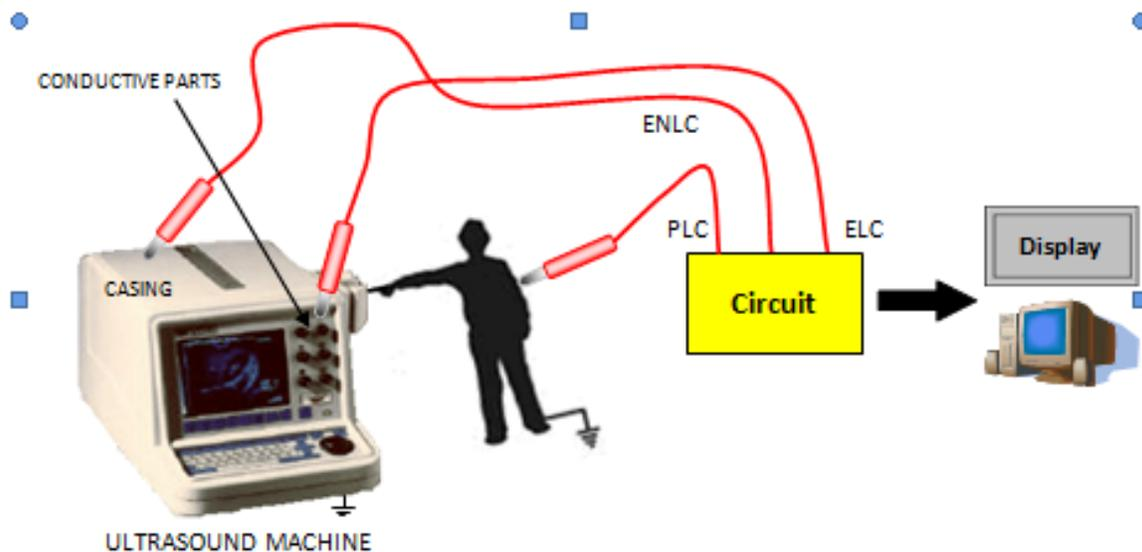
**Figure 6-28 Real Time Leakage Current Monitoring System**
