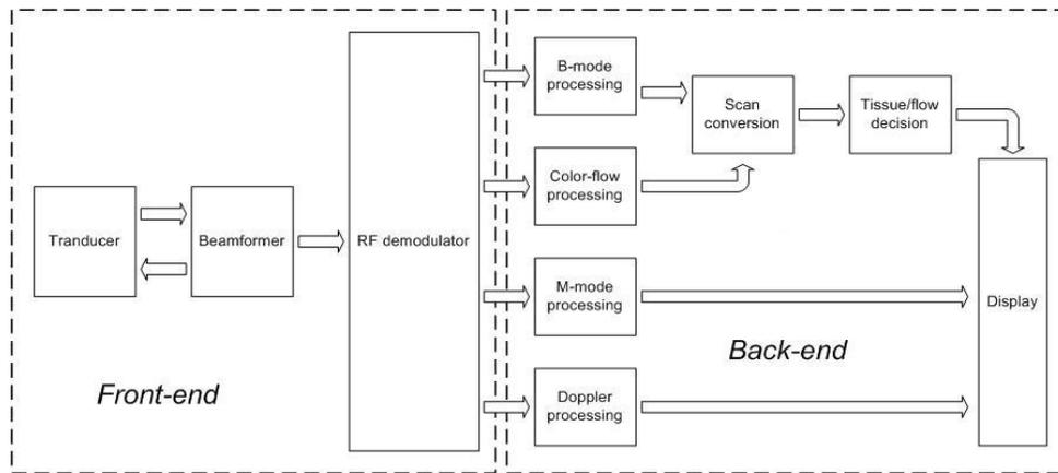
**Figure 4-1 Block diagram of a typical ultrasound machine where the shaded area represents the back-end blocks used in color-flow mode.**
