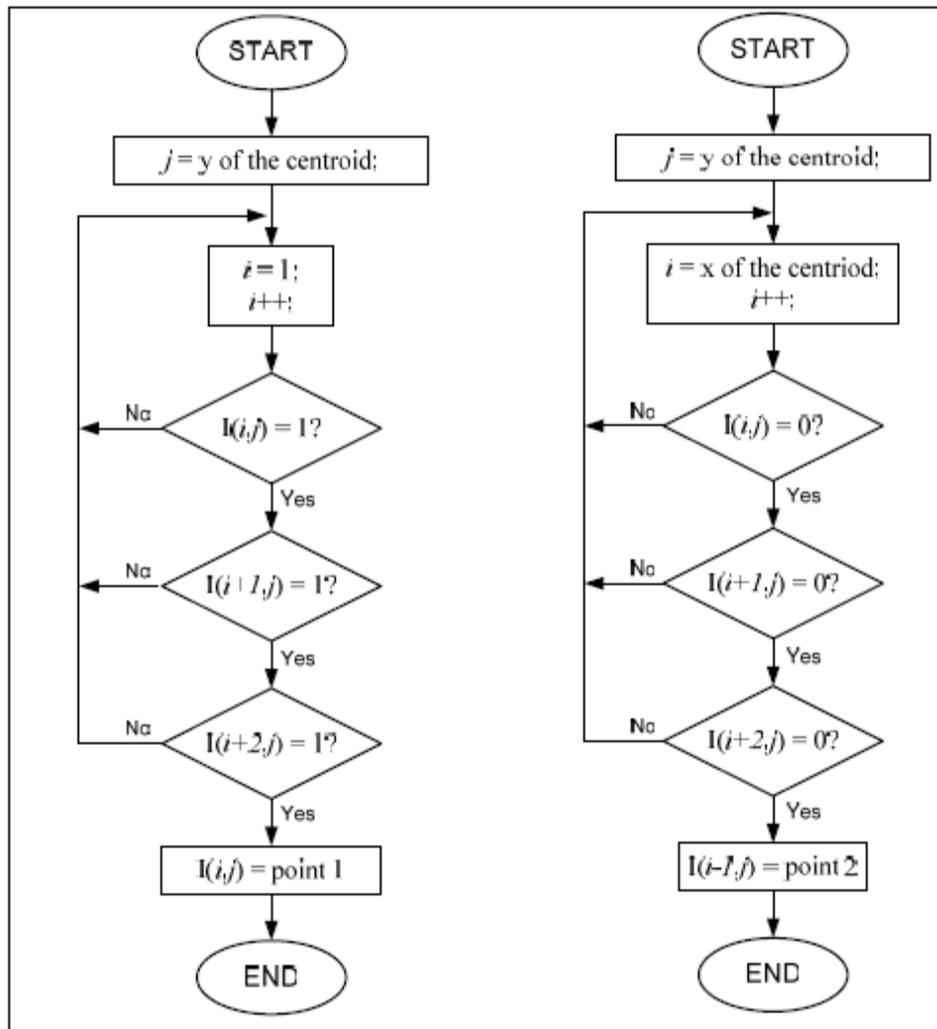
Figure 6-6 Iteration flow for point 1 and 2
