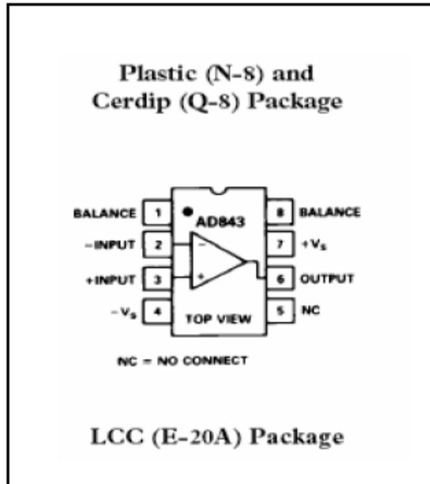
**Figure 6-20 Pin diagram for the AD843 IC**
