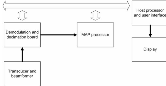
**Figure 4-2 Block diagram of software-based ultrasound machine**
