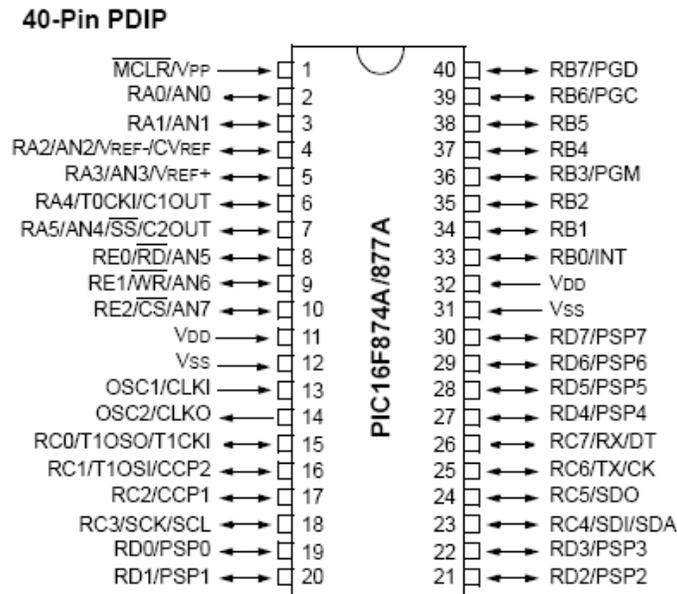
**Figure 6-30 Pin description of PIC16F77A**
