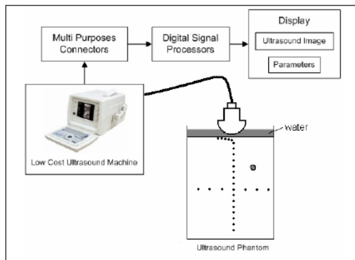
**Figure 6-1 Block diagram of Sonoimprometer**
