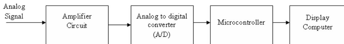
**Figure 6-27 Block Diagram of the leakage current meter**
