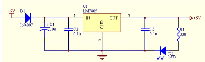
**Figure 6-32 The Voltage Regulator circuit**
