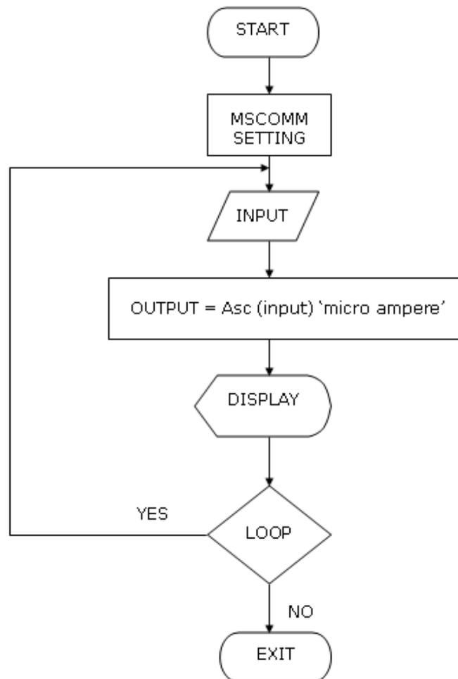
Figure 6-36 Flow chart of the Visual Basic Programming
