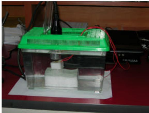
**Figure 6-26 Hydrophone tank**
