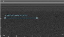
At first endpoint is displayed measurement number ("1:") and measurement result ("HR2b=60 b/min; t=2.000 s"), where 60 b/min is calculated heart rate ("HR") assuming that was measured 2 beats interval ("2b"), t=2.000 s is measured time along x axis.
